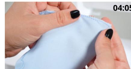
**Sewing:** Overlock all pattern pieces after cutting. Using a sewing machine, use a zigzag stitch with a stitch width of 3.0 and a stitch length of 1.2. An overlock machine can also be used.
